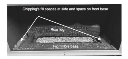
Rear log sits at back in channel as shown ensure air inlet is not blocked
