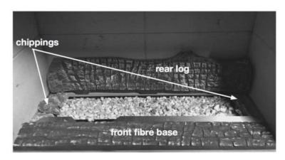
Rear log sits at back in channel as shown ensure air inlet is not blocked Front fibre base sits in front channel as shown cut out underneath to the rear to allow no impingement
