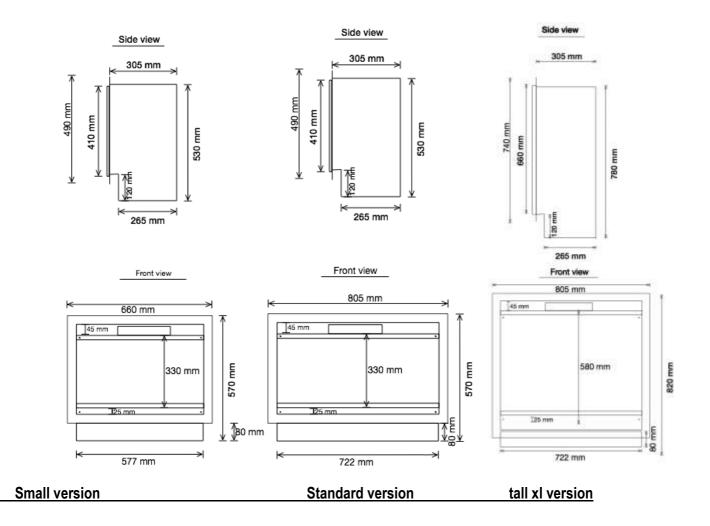
ALL MODELS HAVE A 25mm AIR SUPPLY AT THE FRONT BOTTOM UNDER NO CIRCUMSTANCES SHOULD THIS BE BLOCKED OFF AT ANY TIME
