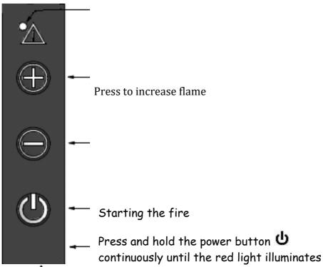
next to the symbol (this takes typically 1 second). As the red light illuminates release immediately the power button. The red light will then flash as the burner is being lit. While the burner is lighting the red light will flash. When the burner has lit the red light will stop completely. The burner will be at maximum burner rate when first lit.
